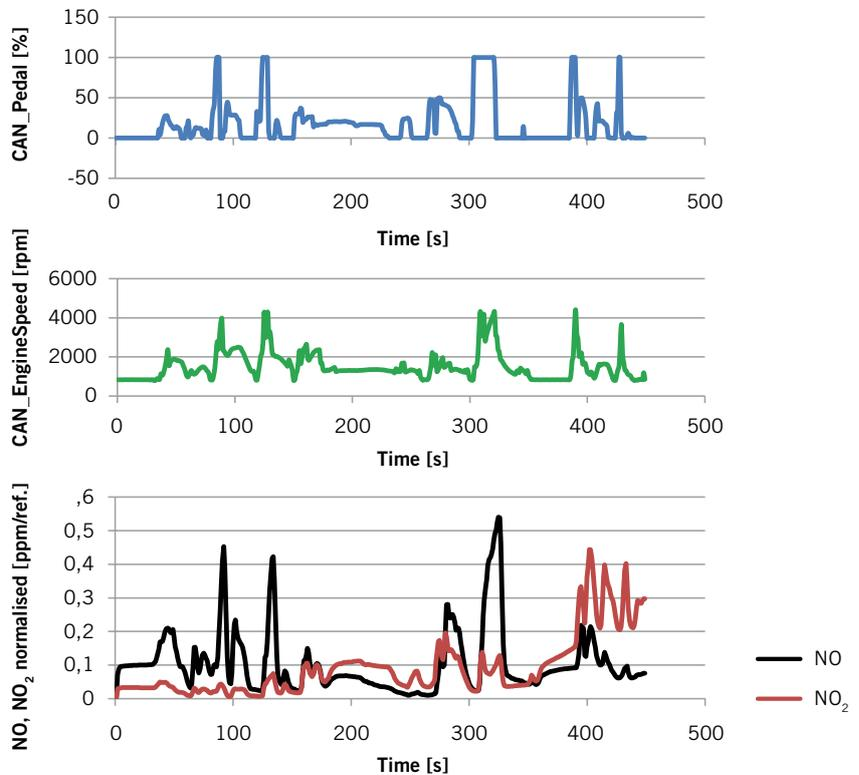
④ Measurement values for pedal position, engine speed and NO/NO<sub>2</sub> emissions; warm vehicle, aggressive driving behaviour (Test 8 in ⑤) – note: NO und NO<sub>2</sub> concentrations (ppm) are normalised, the ratio of NO/NO<sub>2</sub> is correctly displayed
