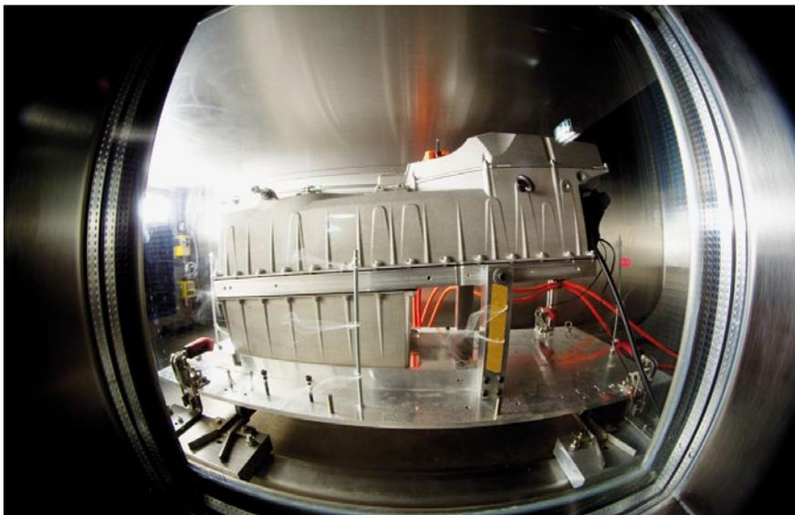
④ High-voltage accumulator in the “accumulator wind tunnel”
