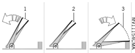
5 The one pedal feeling in three phases braking (1), coasting (2) and accelerating (3)
