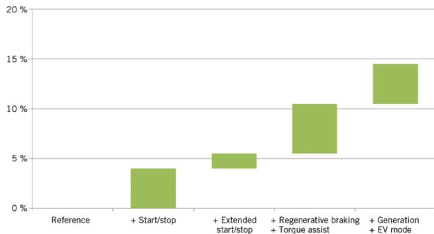
③ Breakdown simulation of CO<sub>2</sub> benefits on NEDC (B-segment gasoline vehicle)
