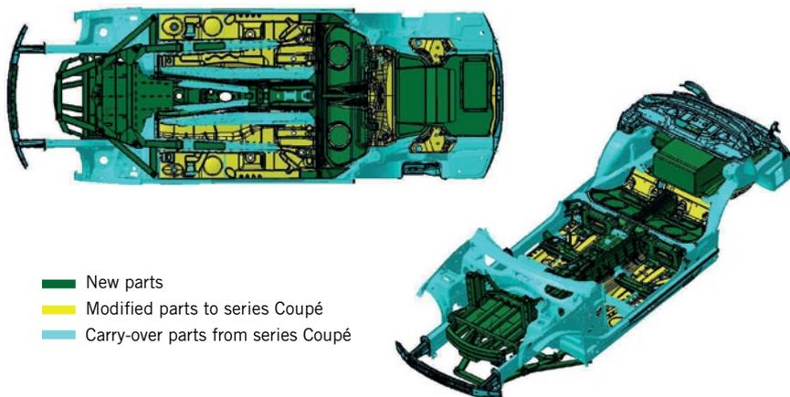
4 New, modified and carry-over parts of the body platform in comparison to the series version BMW 1-Series
