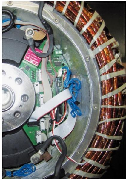
③ In-wheel motor with integrated inverter
