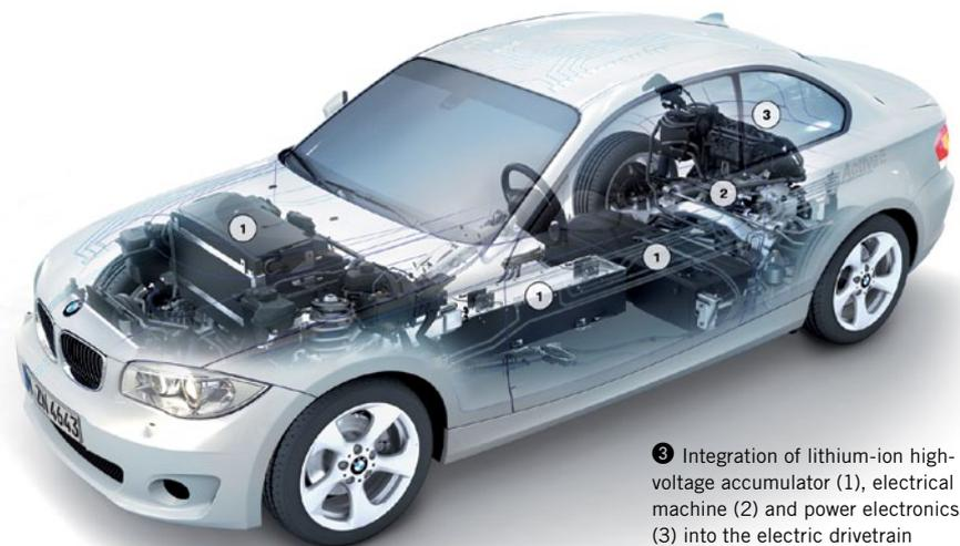
3 Integration of lithium-ion high-voltage accumulator (1), electrical machine (2) and power electronics (3) into the electric drivetrain
