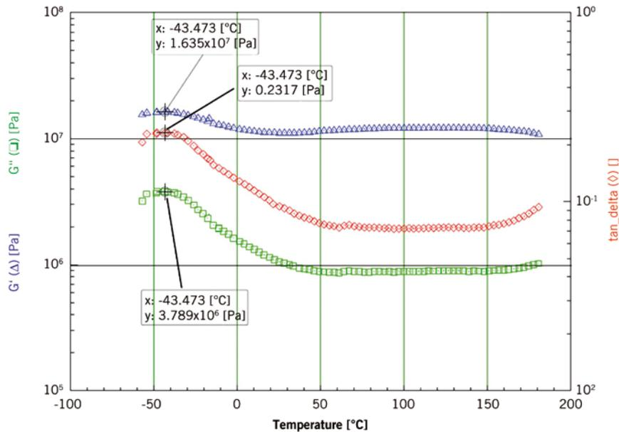
5 DMA analysis of a WarmCure adhesive
