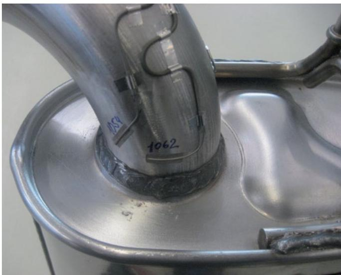
4 Application of the HTSG (two of them with the numbers 1054 and 1062) at the inlet of a muffler
