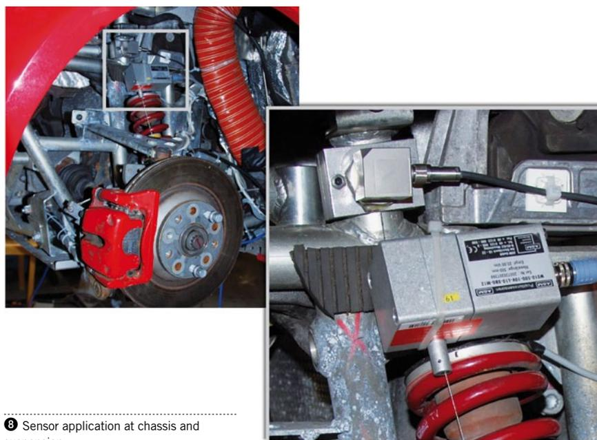
8 Sensor application at chassis and suspension
