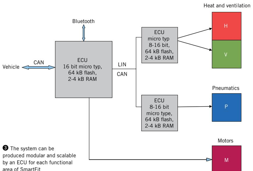
3 The system can be produced modular and scalable by an ECU for each functional area of SmartFit
