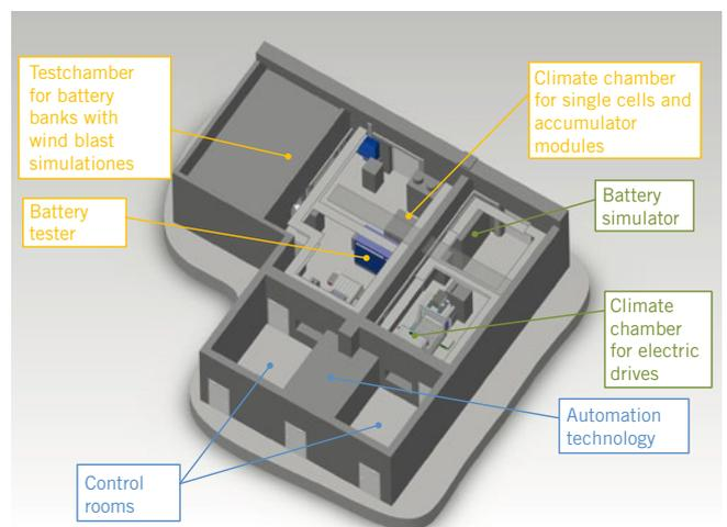
❶ View of the E drive and accumulator test rig
