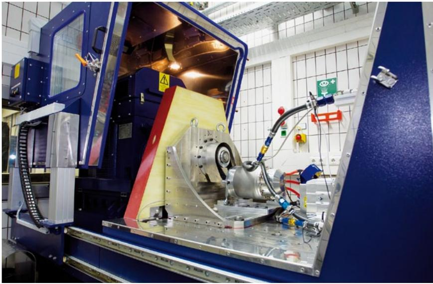
② Electric machine and power electronics in the climate chamber on the E drive test rig
