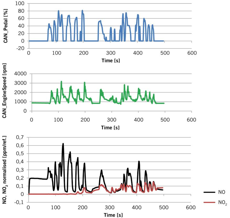
③ Measurement values for pedal position, engine speed and NO/NO<sub>2</sub> emissions; cold vehicle, defensive driving behaviour (Test 2 in ⑤) – note: NO und NO<sub>2</sub> concentrations (ppm) are normalised, the ratio of NO/NO<sub>2</sub> is correctly displayed
