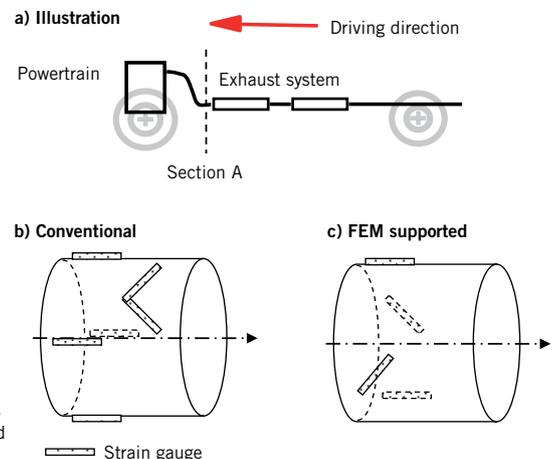
① Comparison of the high-temperature SG application at a pipe: illustration (a), conventional use (b) and FEM supported application (c)
