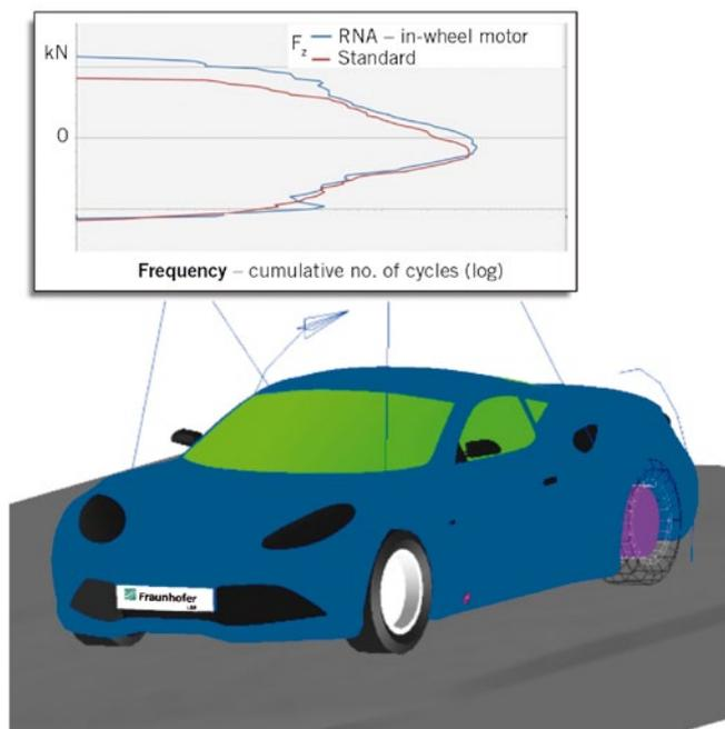
5 Multi-body analyses of complete vehicle structure
