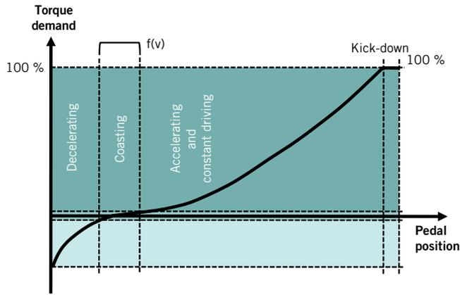
6 Accelerator pedal position and torque demand in the three phases decelerating, coasting and accelerating
