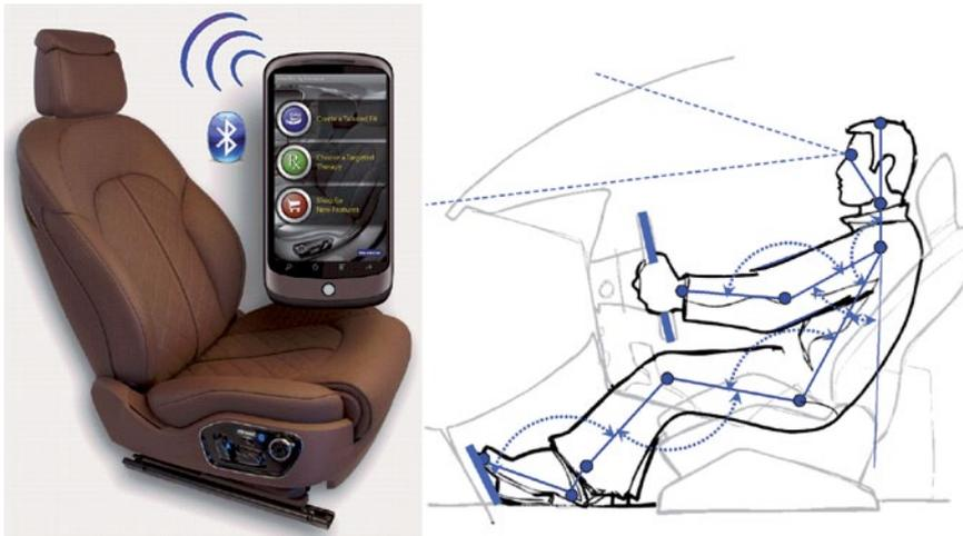
2 SmartFit considers six different angles and twelve different lengths and distances to calculate the optimal seat position
