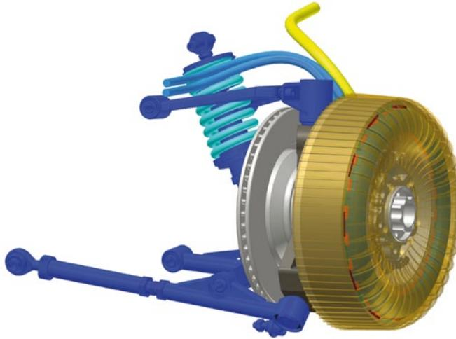
② Study of package of in-wheel motor at rear suspension
