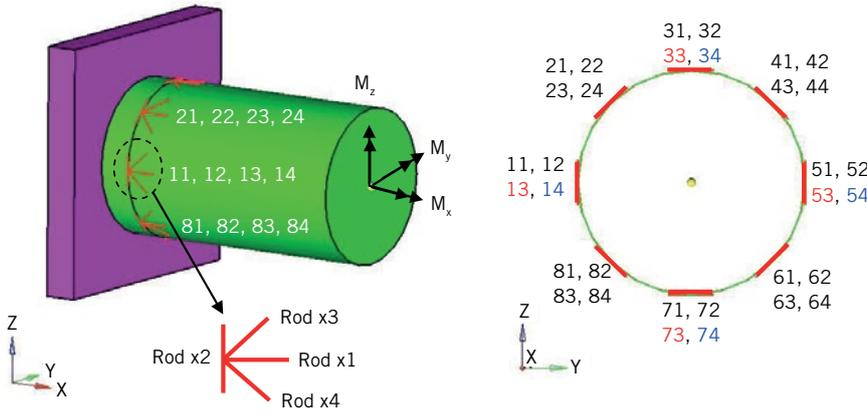
3 Layout of the strain gauges as red bars on a cylinder beam
