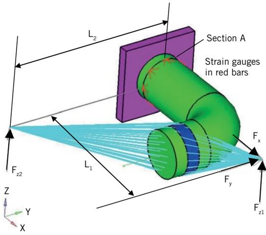
② Static calibration for bending moments, torsion and axial force
