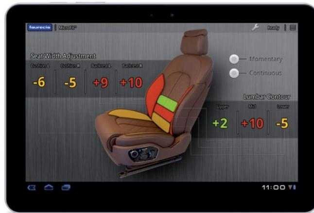
5 When the driver sits down the pressure sensor immediately determines which pneumatic cushion has too much (red), too little (yellow) and right (green) air filling
