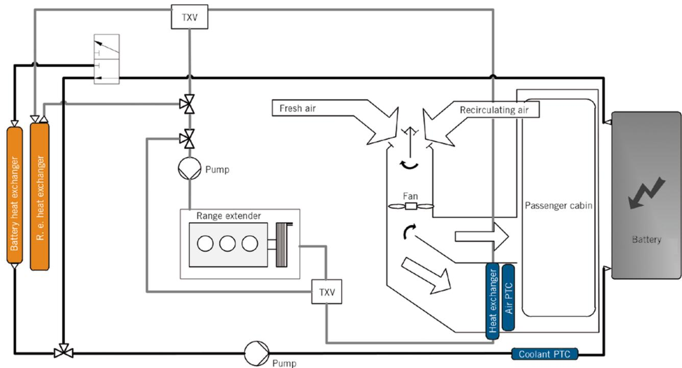
❷ Cooling and heating circuits of the range extender vehicle (TXV = thermostatic expansion valve)
