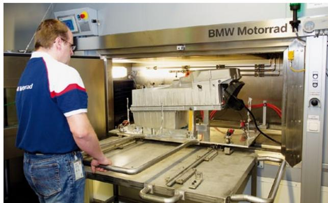
③ Test chamber for battery banks
