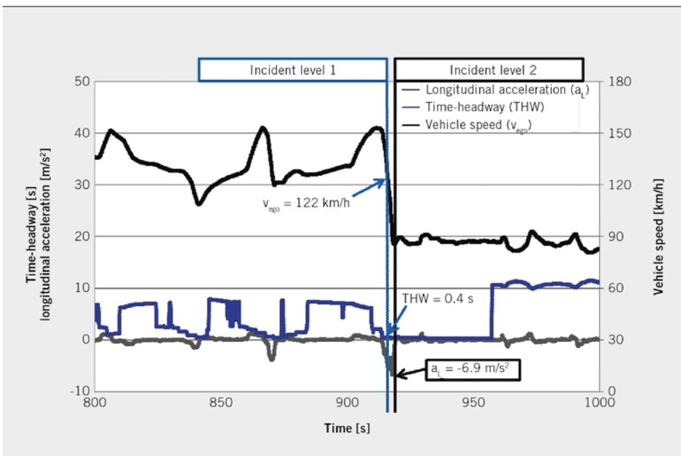
8 Recognition of an incident by means of THW and longitudinal acceleration
