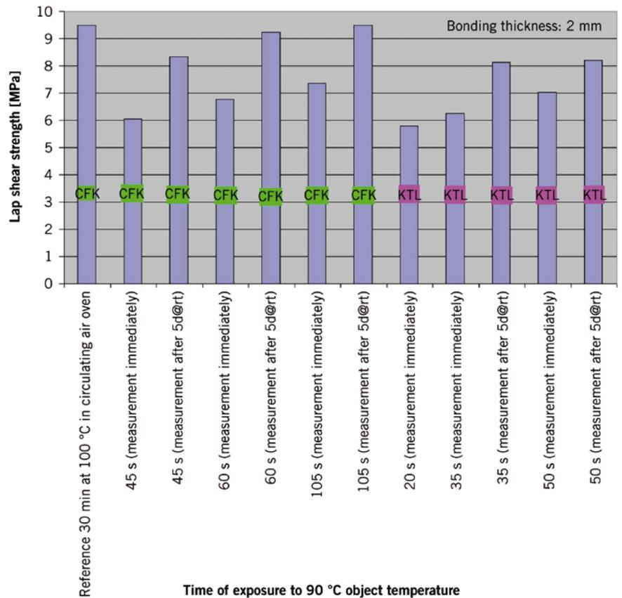
④ Tensile shear strength values as a function of the curing conditions
