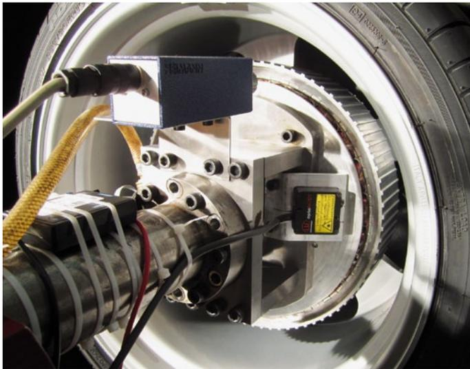
⑨ Laboratory measurement and testing of in-wheel motor
